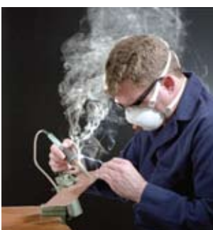
Figure 45 Soldering with and without Tyndall illumination
