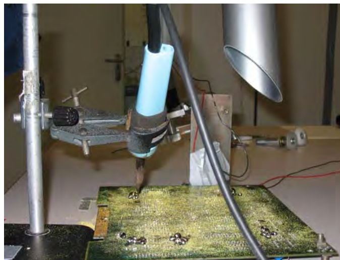
Figure 3.5 Photograph showing condensed solder fume on the PCB and surroundings, also showing the mobile capturing hood in the realistic position. The slot in the soldering iron handle for the tip extraction nozzle can be seen just to the right of the mains cable.
