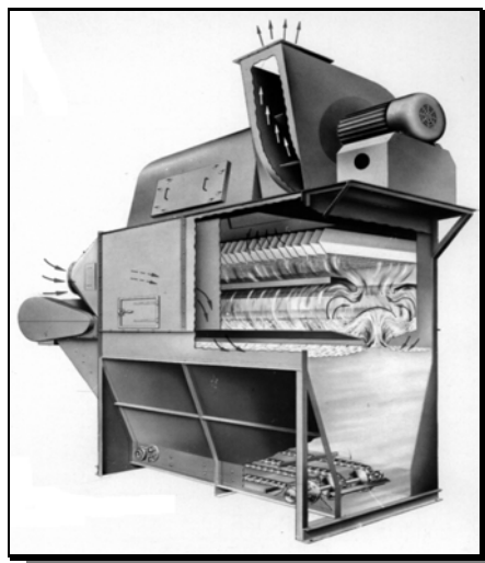
Fig.6 Induced Spray Wet Collector
